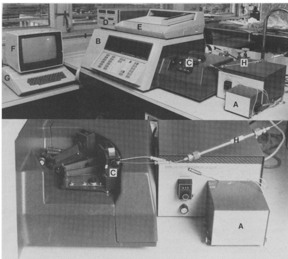
Fig. 1. UV-visible detection set-up used in the HPLC experiments.
